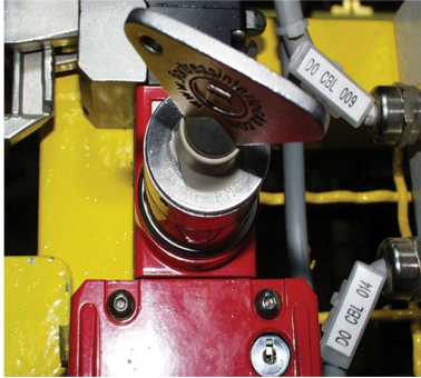
SBS1LOK ; solenoid controlled safety gate switch with safety key and sidebar
